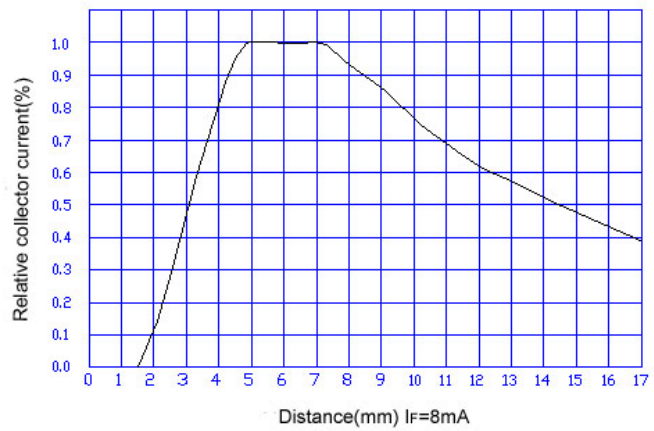
Fig.2 Relative collector current vs. distance
